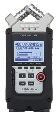
MODE and pressing the dial. Your options are either Stereo (which records either the XY mic on top of the device or the XLR inputs on the bottom to a single stereo file), 4CH (which records both the XY mic and the XLR inputs to two separate stereo files) or MTR mode (which allows for multitrack recording).
